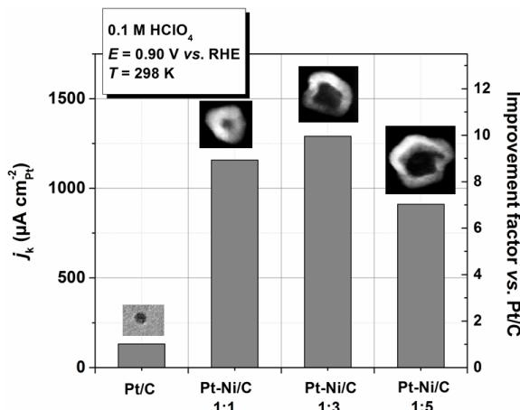
Changes of the ORR specific activity on porous hollow Pt-Ni/C nanoparticles with different structural and chemical properties. A 10-fold improvement is obtained over standard Pt/C nanocrystallites.
