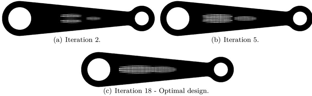
Figure 3.5: Topology evolution of the connecting rod.
