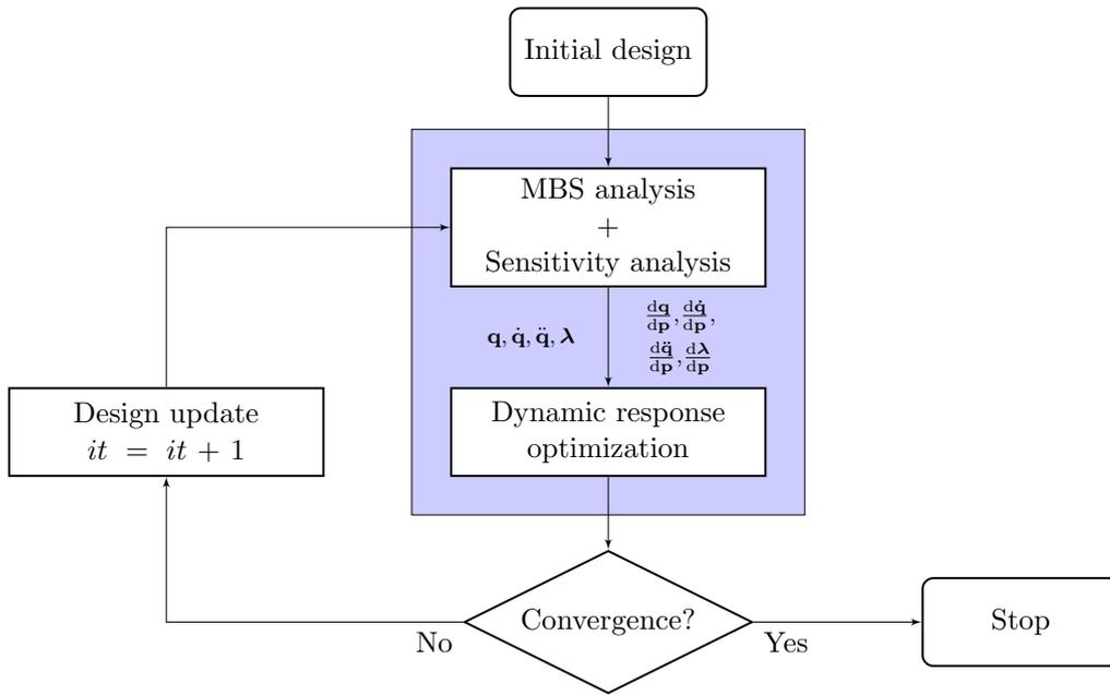
Figure 3.6: Fully coupled method framework.
