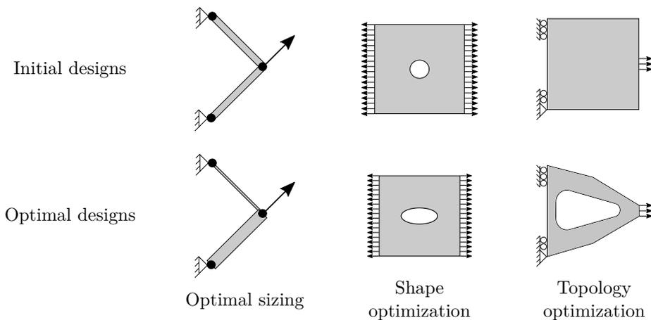
Figure 2.5: Structural optimization parameterizations.
