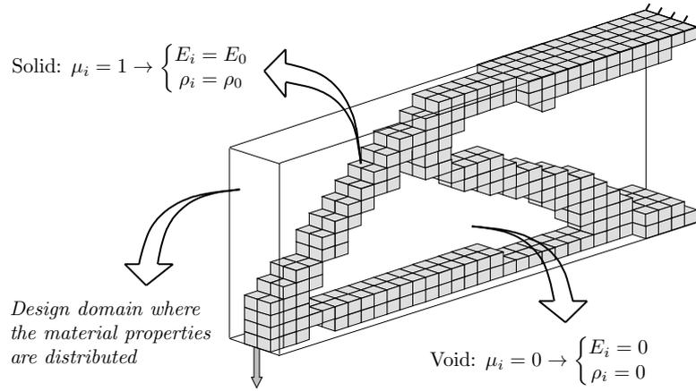
Figure 2.6: Optimal distribution of material in topology optimization (Duysinx and Bruyneel, 2002).
