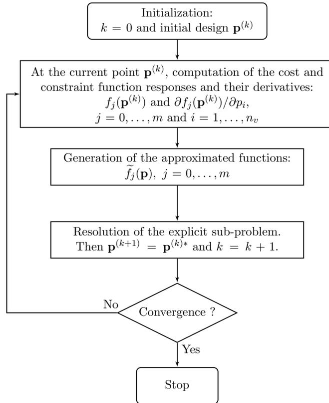
Figure 2.8: Iterative process of the sequential convex programming method (Bruyneeel et al., 2002).
