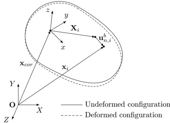
Figure 3.9: Description of the deflection of node  $i$  in body  $b$  with respect to a corotational frame.
