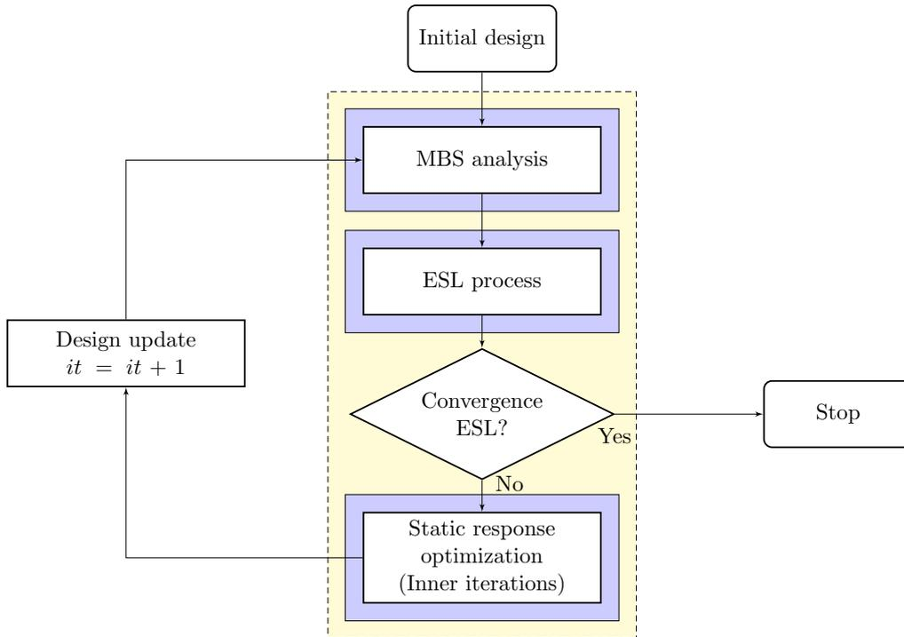
Figure 3.11: Weakly coupled method framework.
