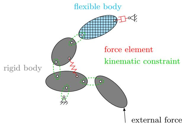
Figure 2.1: Multibody system diagram.
