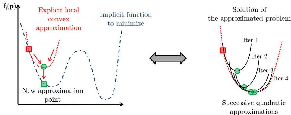
Figure 2.7: Sequential convex programming approach.
