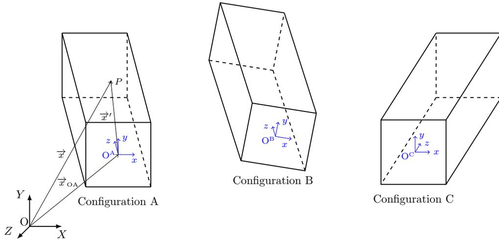
Figure 2.4: Free 3D motion of a single rigid body represented at three different configurations.
