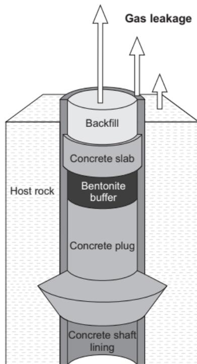
**Figure:** Layout of the sealing system used for the shaft n°6 of Anderlues coal mine.
