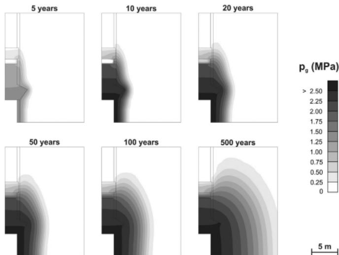
**Figure:** Evolution of gas pressures in the different materials during  $CO_2$  storage in the coal mine.
