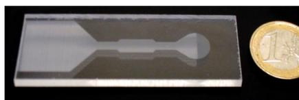
Laser ablated PMMA slab
