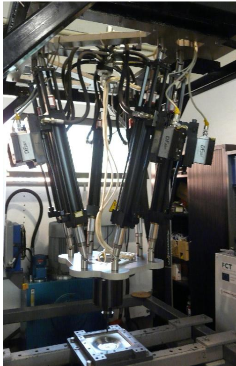
Figure 1.6: Prototype machine for SPIF from University of Aveiro.
