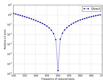
The ROM is constructed with an interpolated reduced basis. The interpolation uses two basis around 350Hz. The first reduced basis  $\Psi_1$  is fixed from solution at 320Hz. The second one  $\Psi_2$  is varying from 351Hz to 380Hz.
