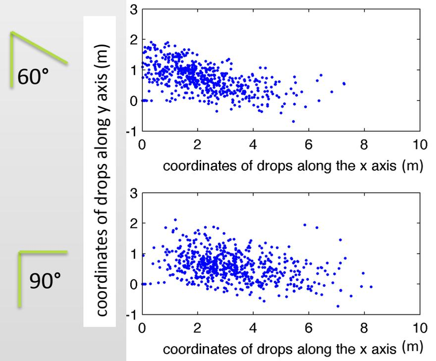
**Hydraulic nozzle:** VMD=270  $\mu\text{m}$ ; Span=1.1 Emitted droplet velocity= 10 m/s
