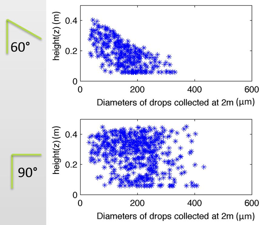
**Hydraulic nozzle:** VMD=270  $\mu\text{m}$ ; Span=1.1; Emitted droplet velocity= 10 m/s
