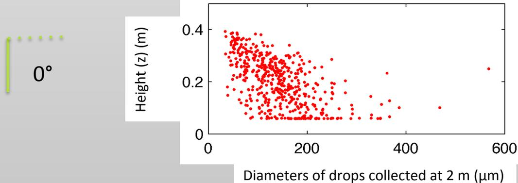
**Rotary atomiser:** VMD=270 ; Span=0.69 ; Emitted droplet velocity= 25 m/s
