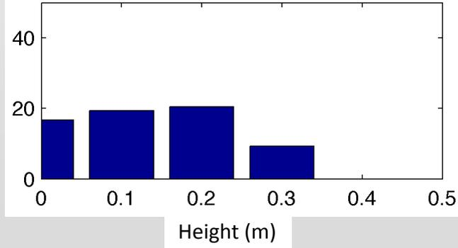
**Hydraulic nozzle:** VMD=270; Span=1.1; Emitted droplet velocity= 10 m/s
