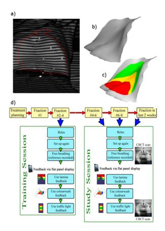
Figure 1 - Showing (a-c) the method of operation of the surface measurement device and (d) the clinical trial protocol. The sensor projects a fringe pattern onto the patient (a), analysis of the modulation of which yields the body topology (b). Deviation of the surface from its ideal is displayed as a colour-wash over the live surface (c) or in more abstract format (d).
