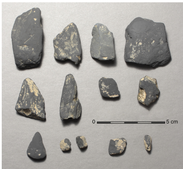
Fig. 6. The BPS fragments have the same macro- and mesoscopic properties: a fine grained, dark grey, and porous siltstone.
