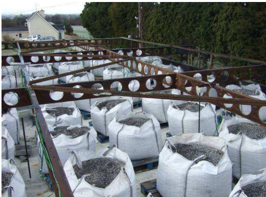
Fig. 3. a) Vertical static load, b) Wooden cribs used for the fire load
