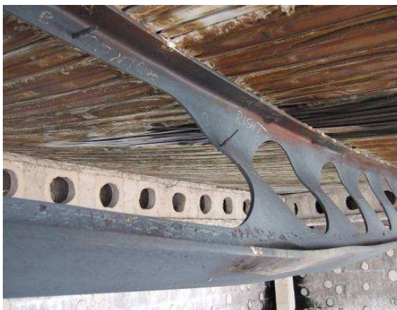
Fig. 7: a) post web buckling , lateral and torsional effect, b) temperature distribution at the steel cross section
