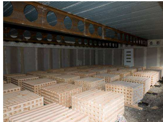
Fig. 3. a) Vertical static load, b) Wooden cribs used for the fire load
