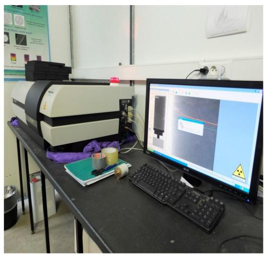
Skyscan-1172 high-resolution desktop micro-CT system (Skyscan, Kontich, Belgium) Image pixel size of 27.27 µm Rotation step was 0.3° over 180° The cone beam source
