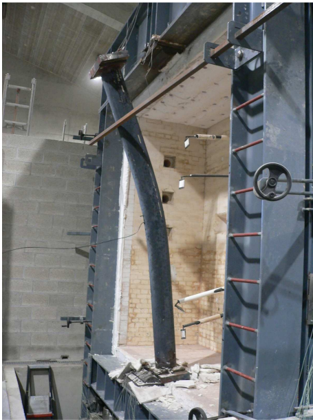
Fig. 2 Column 1A after the test
