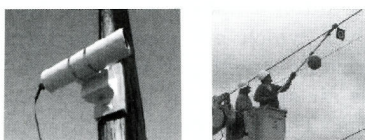
Fig. 13: optical measurement of sag with a camera and a target
