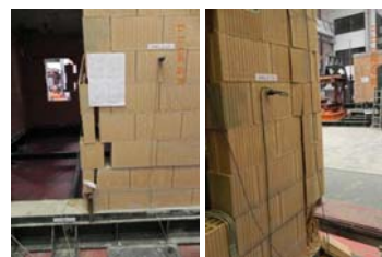
Figure 6. Local crushing of the Mock-up B
