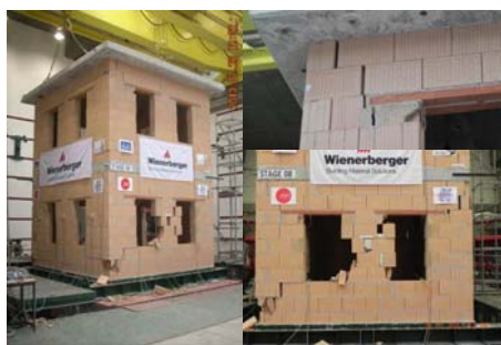
Figure 5. Collapse of the Mock-up B
