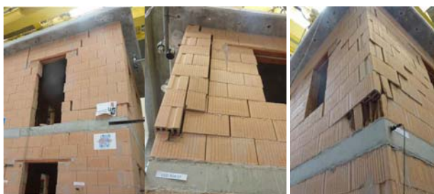
Figure 4. Collapse of the Mock-up A
