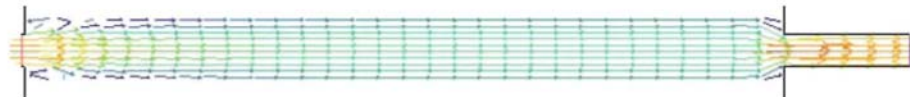
Fig. 13 How field simulated with a uniform specific discharge profile at inflow for the 3 m:4 m basin (algebraic turbulence closure). Velocity magnitude in m/s
