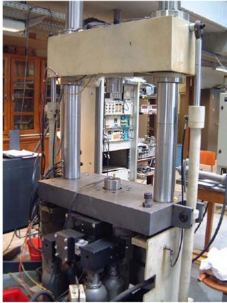
Figure 4-6 Overview of the uniaxial SCHENCK Hydropuls 400 kN machine
