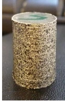
Figure 4-40 Specimen with a stochastic pattern on the lateral free surface
