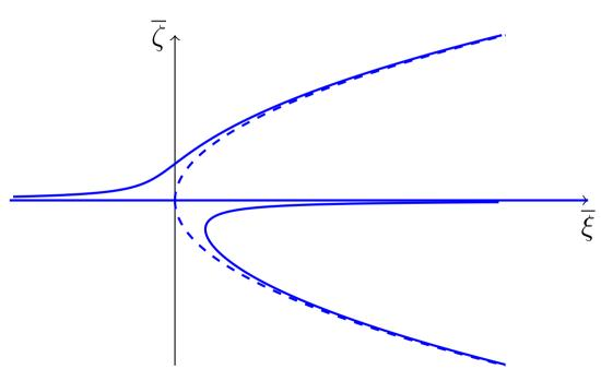
For small-magnitude random imperfection, as  $\epsilon \to 0$ , the bifurcation equation remains random. The random bifurcation diagram is randomly perturbed about the classical pitchfork. The random critical buckling load is always greater than the critical buckling load for the perfect beam.
