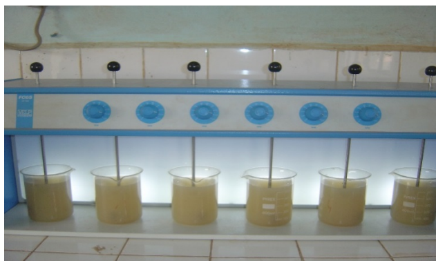
Figure 4. Jar test for water sample clarification (Kaboré et al. [6]).
