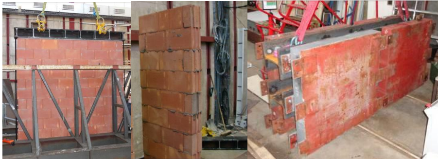
Figure 6. Specimens of the first set (left and middle) and additional mass (right)
