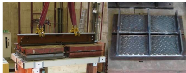
Figure 7. RC slab and steel connectors
