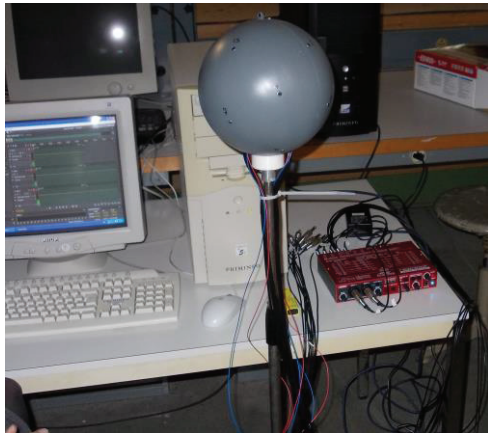
Figure 1. The spherical array with some of its numbered microphones [5].
