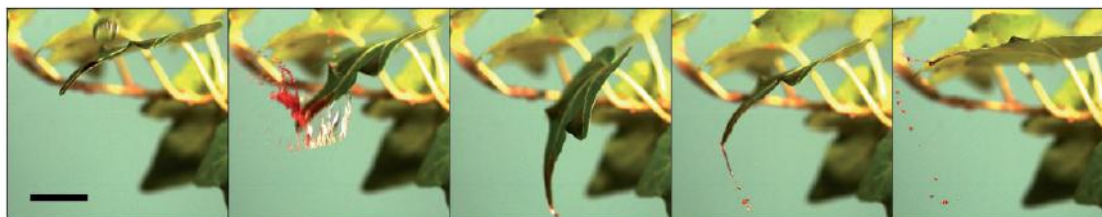
Fig. 6 Coexistence of splash, dripping and catapult during a single impact of a raindrop (diameter 4.6 mm, speed 6.5 m/s) on an English ivy leaf. We=2780 and K=35,000 . Snapshots are taken at impact, then 3, 25, 35, and 45 ms later. The largest droplet ejected by splash and detachment are 0.68 and 0.84 mm in diameter, respectively. Scale bar is 1 cm.
