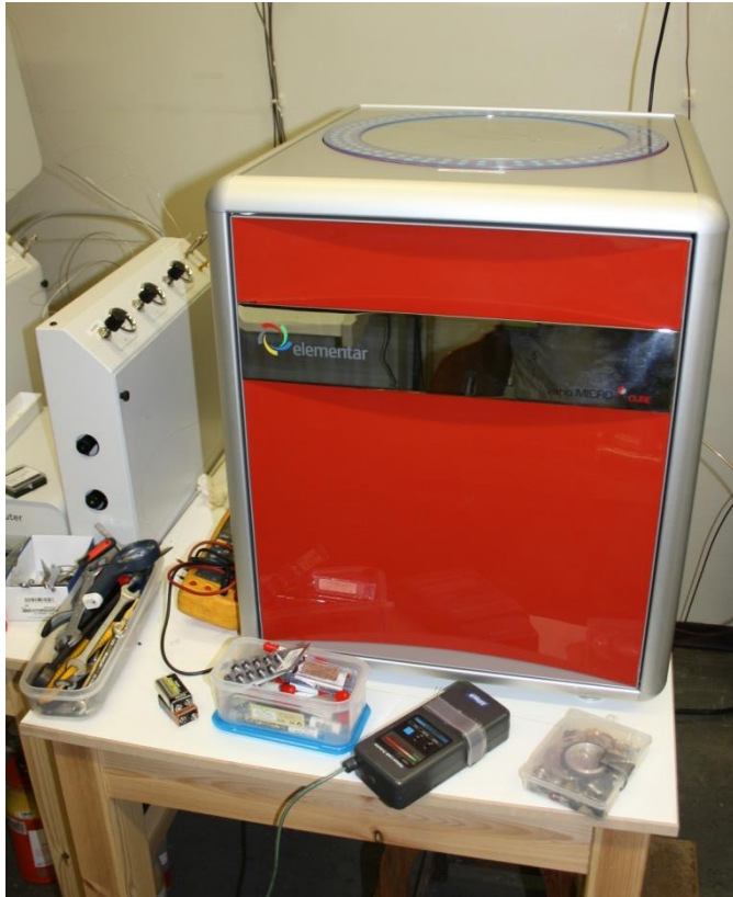
Elemental Analyser (VarioMicro cube, Elementar, Germany)
