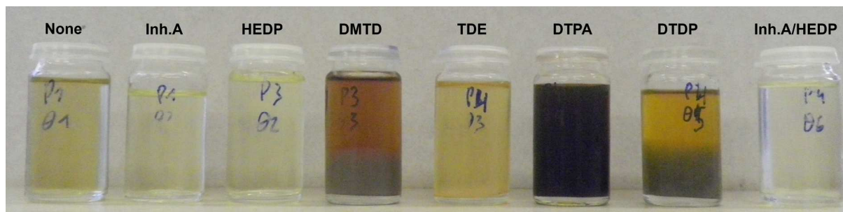
10 11 12 13 14 15 16 17 18 19 20 21 22 Figure 7. Influence of oxidative degradation inhibitors on the color of the degraded solution (100 23 24 g, 30 wt% CO 2 loaded MEA, no gas feed, 140°C, 3 weeks). 25 26 27 28 29
