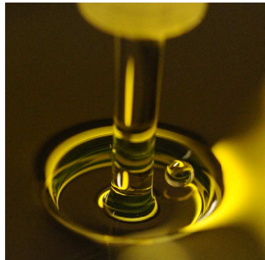
Fig. 1: (Colour on-line) A drop of radius a = 1 mm of silicone oil in non-coalescence state inside a horizontal hydraulic jump of the same liquid ( R = 5 mm).
