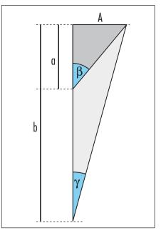
Figure 7 Decrease of angular opening with length of the osteotomy.  $\gamma$  is smaller than  $\beta$  as the distance b is longer than a.
