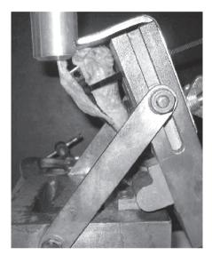
**Figure 5** Axial loading of the tibial crest via load applied that is perpendicular to the tibial plateau. The patella was fixed in a rigid split cup connected to the cross-bar of the servohydraulic testing machine and axial load was applied to the tibial tuberosity via the patellar tendon.
