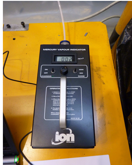
(b) Mercury vapor detector: detection above 3 feet from the ground (range 1-2000 \mu\text{g}/\text{m}^3 ).
