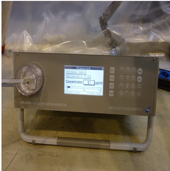
(a) Mercury vapor monitor VM-3000: detecting on the ground surface just below the mirror.
