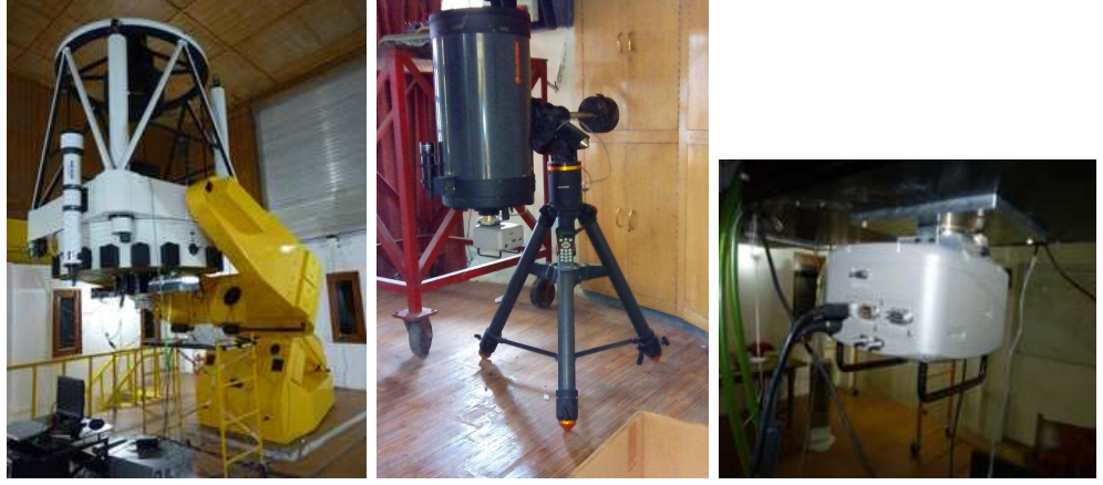
Figure 6.15: TDI set-up at the 1.3m DFOT and C-14" telescopes. From left to right: SBIG camera installed at the focal plane of both telescopes and zoomed image of the SBIG CCD at the DFOT.
