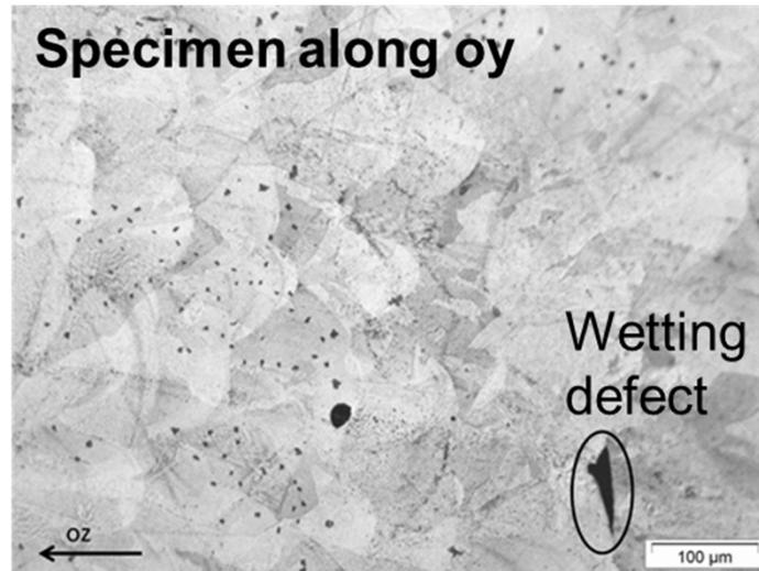
Deterioration of the mechanical properties for the oz specimens due to their **higher volume fraction of defects** and to their very **detrimental orientation** (i.e. perpendicular) with respect to the loading direction
