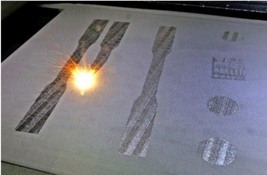
Laser Beam Melting
