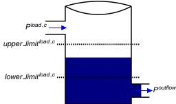
The **tank model** for representing loads with inner storage capabilities: the power consumption of the load  $P^{load,c}$  (inflow of the tank) can be modulated under the constraint the level of the tank stays within its limit.  $P^{outflow}$  is the (uncontrollable) outflow of the tank.
