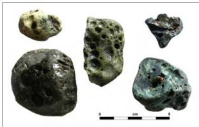
Fig. 1. Rounded vitreous iron slag found in the Lembrée River (Ardenne)
