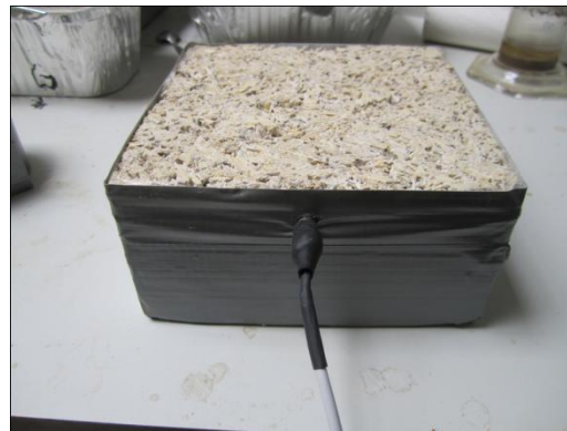
Fig. 2. LHC bloc with sealed lateral faces
