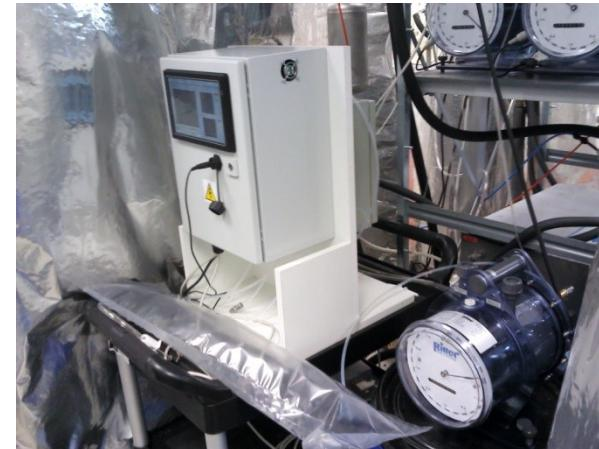
**e-nose** = array of 6 low-specificity gas sensors
