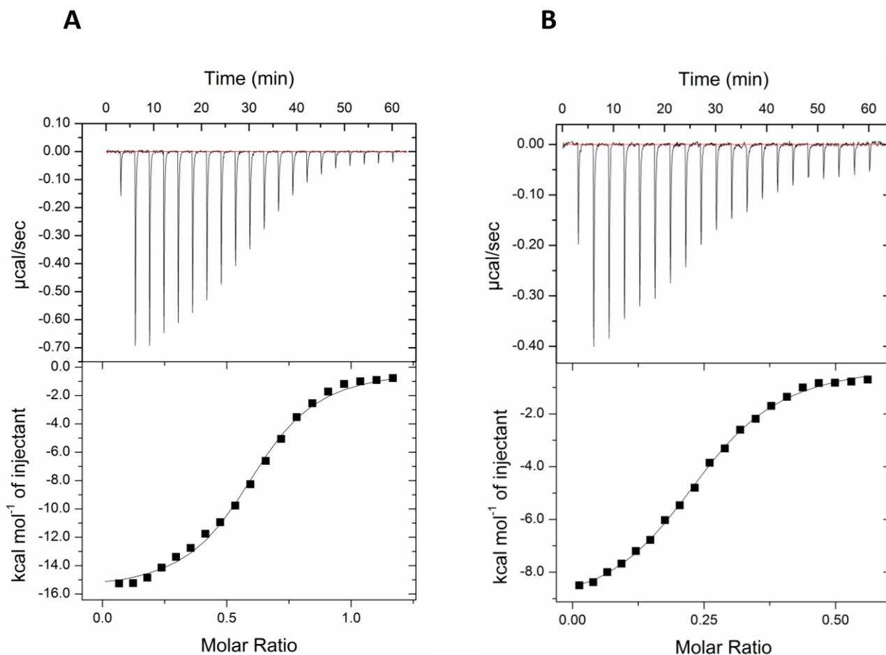
**Supplementary Fig. S4.** Isothermal titration calorimetry of TFs binding to  $\alpha$ -casein in direct titration. Upper panel: exothermic microcalorimetric traces of  $\alpha$ -casein injections into TFs. Lower panel: Wiseman plot of heat releases versus molar ratio of injectant/protein in the cell and nonlinear fit of the binding isotherm for  $n$  equivalent binding sites.
