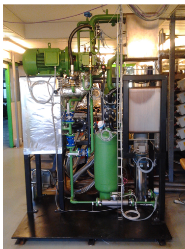
(a) Front view of the ORC test rig
