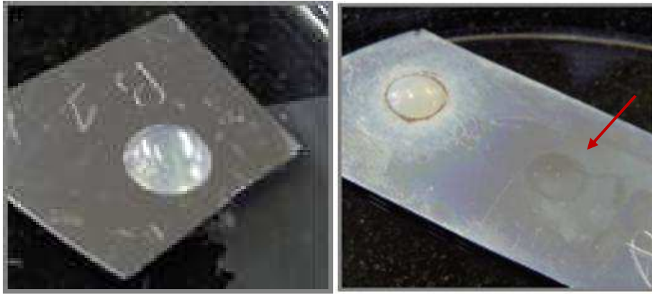
Fig. 3: The encapsulant before release (left), and after release (right), the droplet (on the right part of the image) is peeled off during the release, whereas the droplet (on the left of the image) remains on the surface, hence delamination and microcracks are visible.
