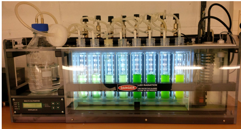
Figure 1. Cultivation of Chlorella in a tube photobioreactor.
