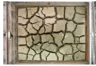
Fig. 6 Cracks network on the surface of the Romainville clay after drying from Ta (2009)
