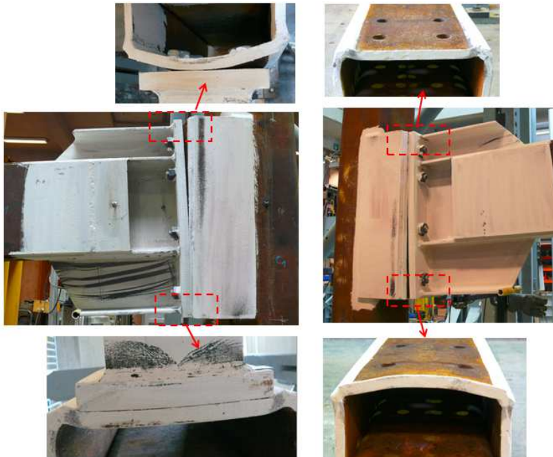
Figure 9: failure mode of the B-EP-U joints (reverse U channels yielded)
