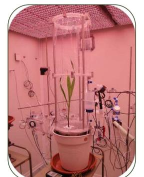
Chamber cuvette (44L) for PTR-MS and GC-MS measurements (BISA)
