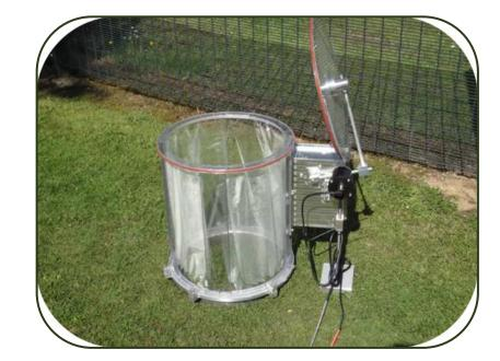
Field cuvette (22L) for PTR-MS and **GC-MS measurements (BISA)**
