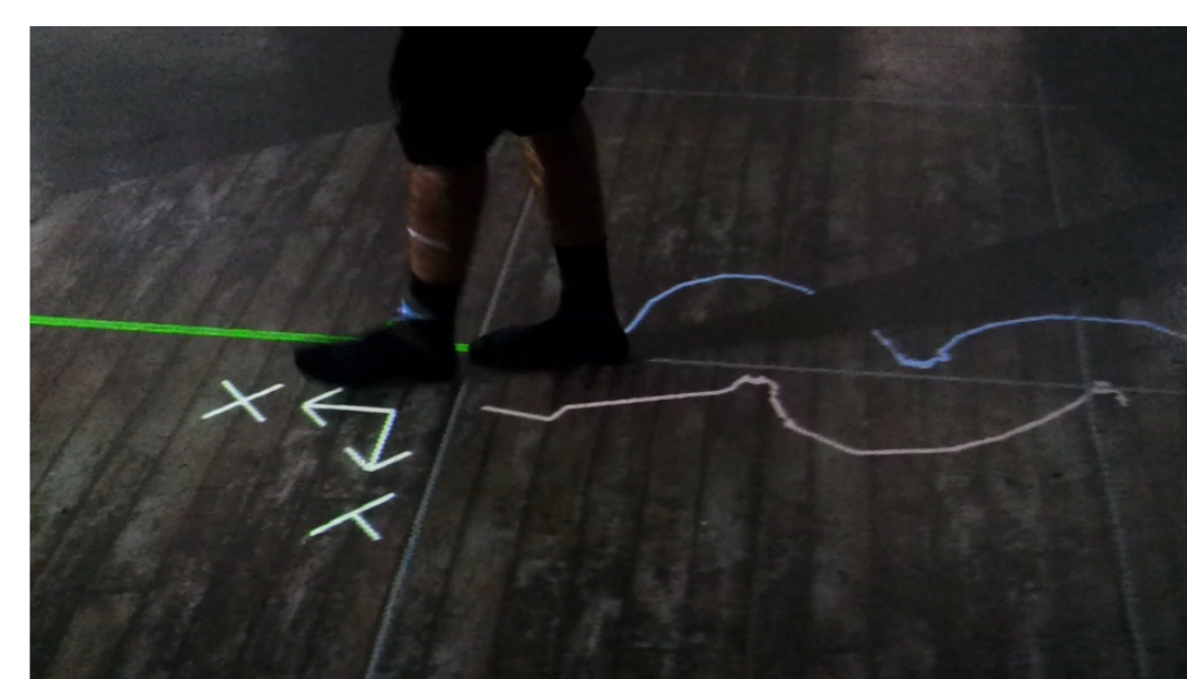
(b) This picture shows the path followed by the patient in green, and the measured feet trajectories projected in real-time on the floor using a beamer.
