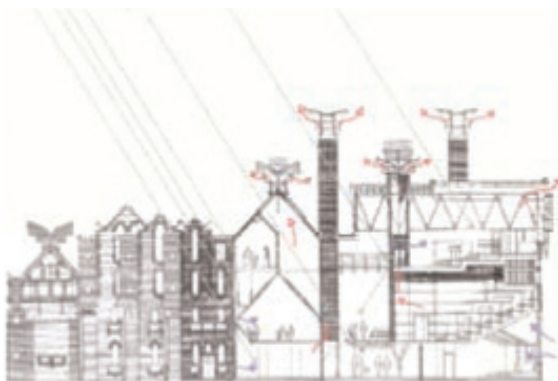
Fig. 4.45, Natural ventilation as Icons (De Montfort University, UK: Short Ford & Associates, Architects).
