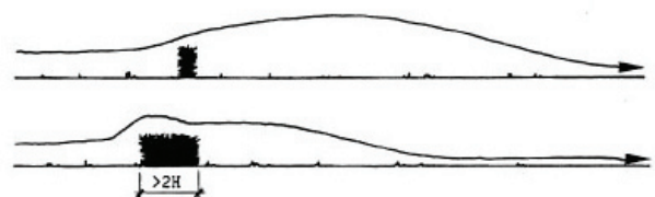
Fig. 4.70, Effect of the along wind depth of windbreaks on the sheltered area (Arens and Watanabe, 1986).
