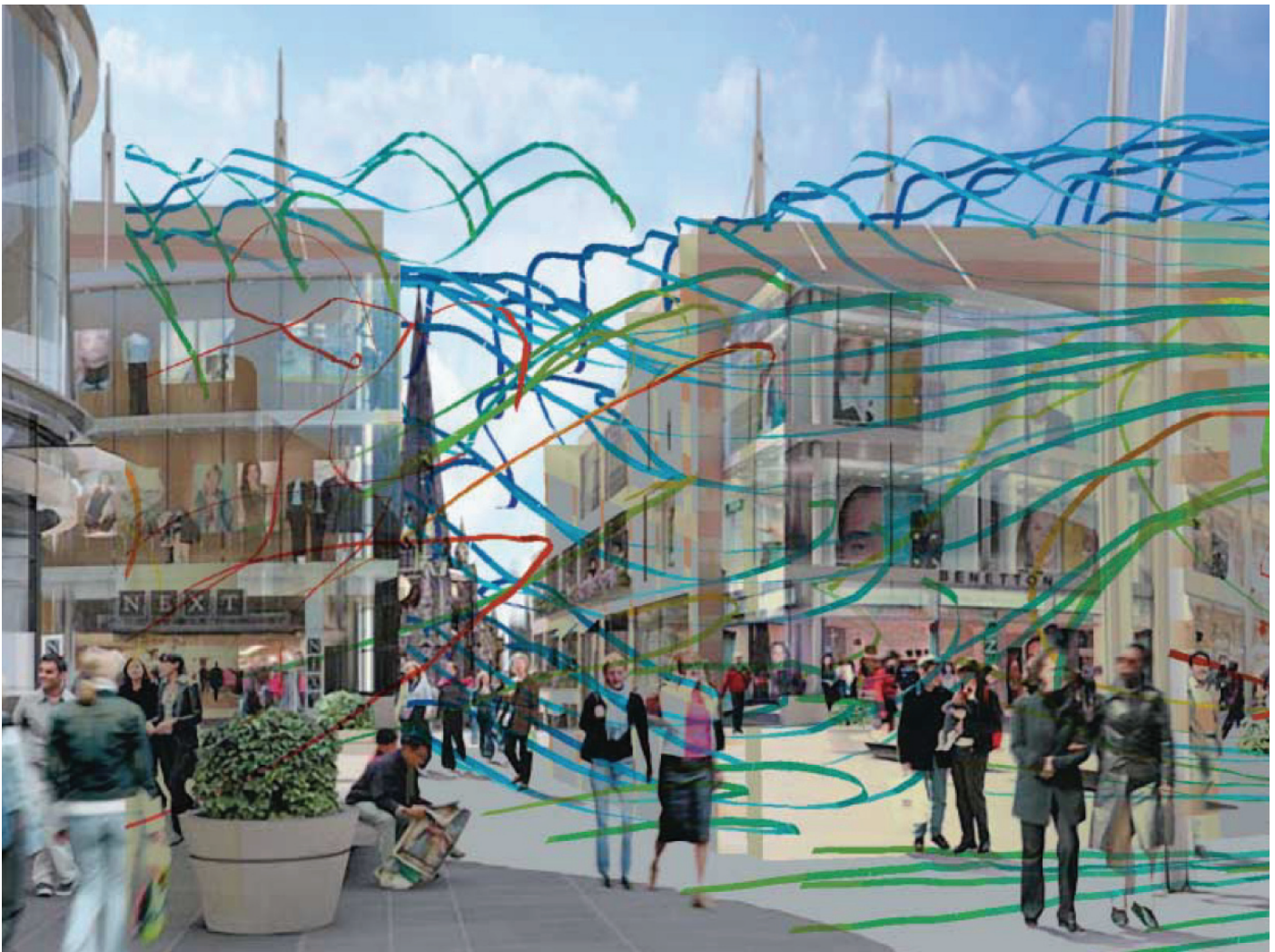
Fig. 6.05, Artist's impression of Bullring in Birmingham, England, with superimposed CFD prediction of outdoor wind floor path lines coloured by local flow velocity.
