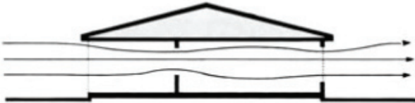
Fig. 4.42, Wind-driven ventilation (Abdel Halim CDC and Sasaki Associates, 2000b).
