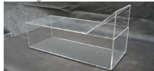
Fig.5, Plexiglas model was constructed to allow multiple settings, scale 1:20.
