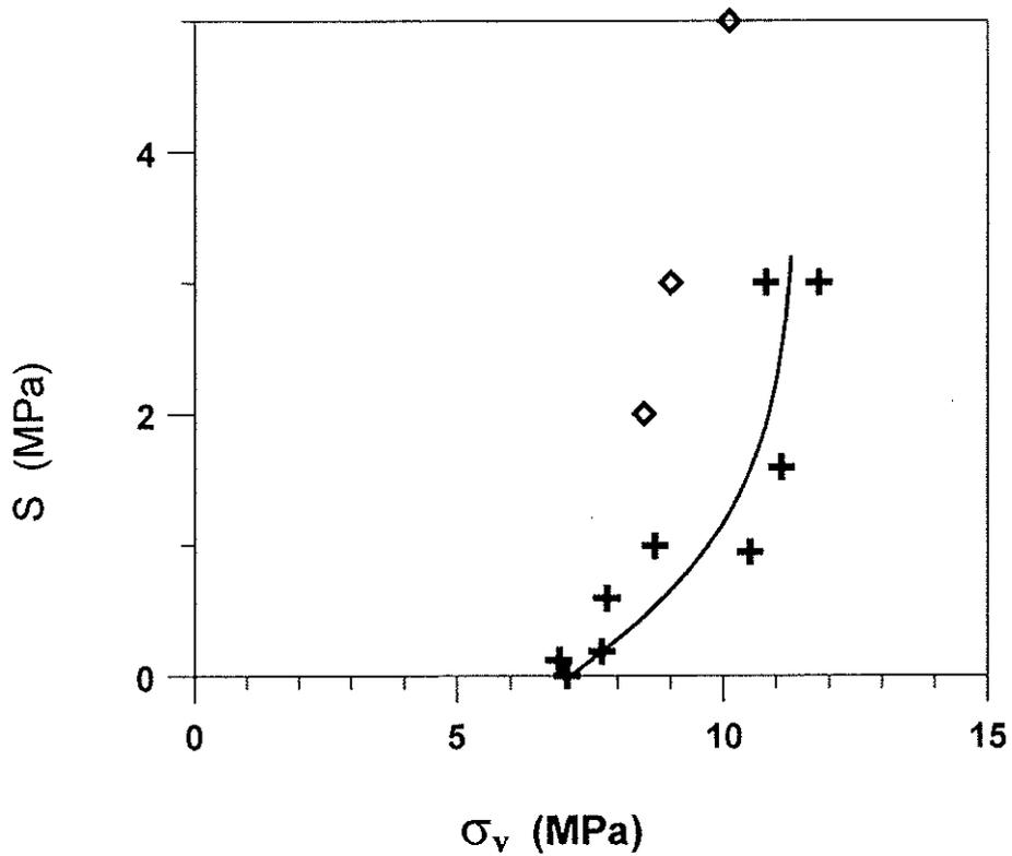
Figure 4: Effect of suction on the preconsolidation pressure – relationship  $P$ - $\sigma_{v0}$ .
