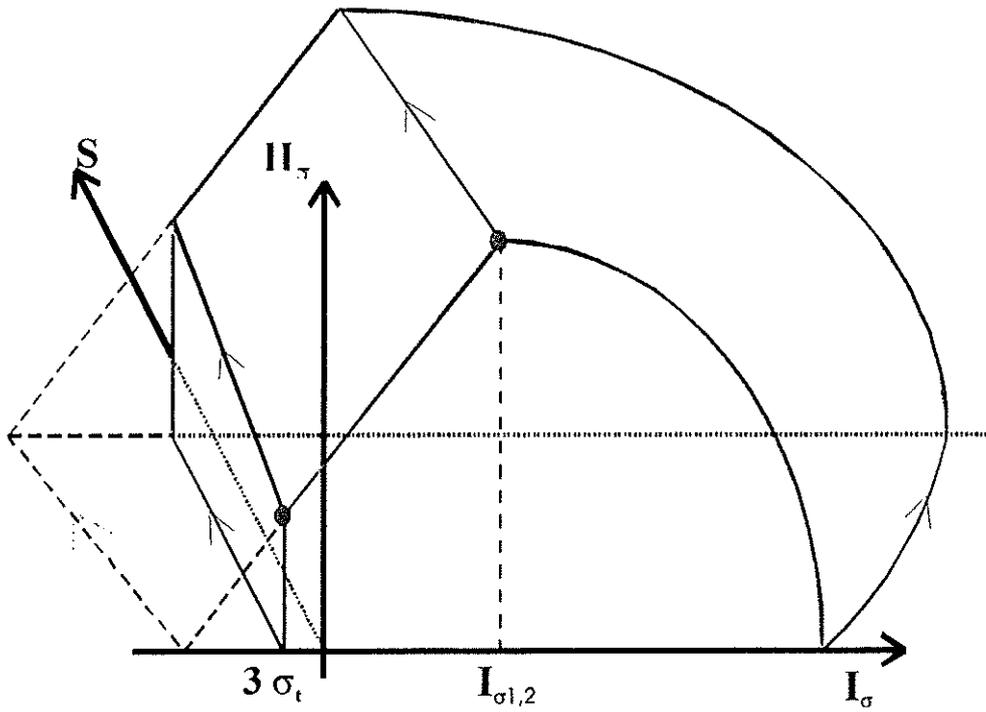
Figure 1: Cap model in the  $(I_\sigma, II_\sigma, s)$  space, soil and rock mechanics sign convention
