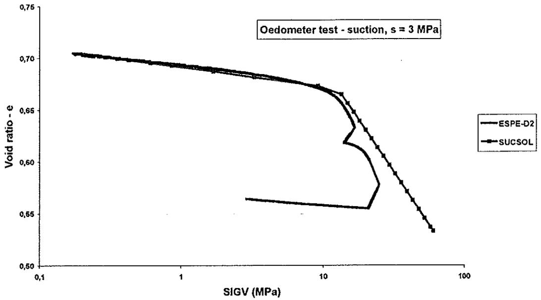
Figure 8: Simulation of an oedometric test
