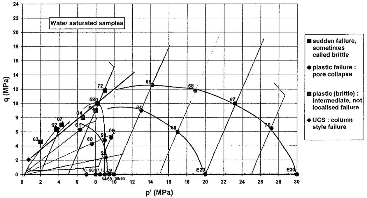
Figure 5: Test on water saturated chinks – Stress paths and failures points
