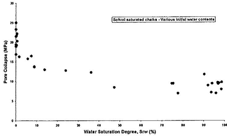
Figure 7: Hydrostatic tests - collapse function of initial water saturation degree
