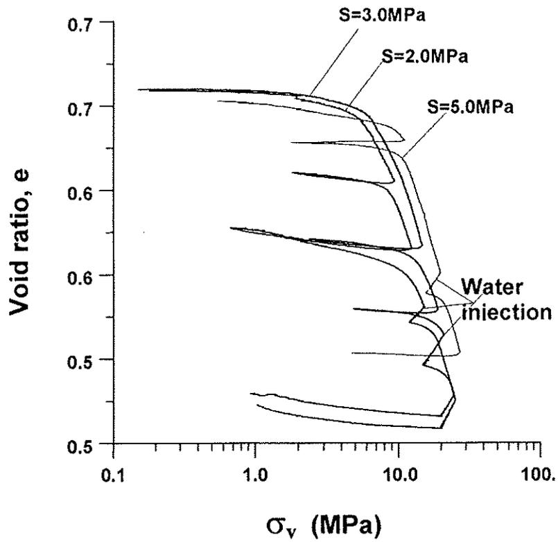
Figure 3: Oedometer tests at different suctions in  $e$ - $\log \sigma_v$  plan.
