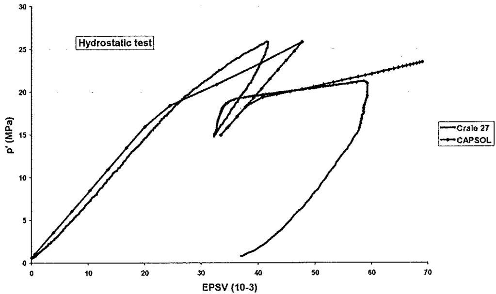
Figure 9: Simulation of an hydrostatic test
