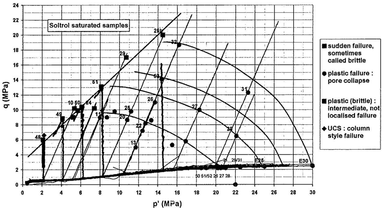
Figure 6: Test on Soltrol saturated chinks – Stress paths and failures points
