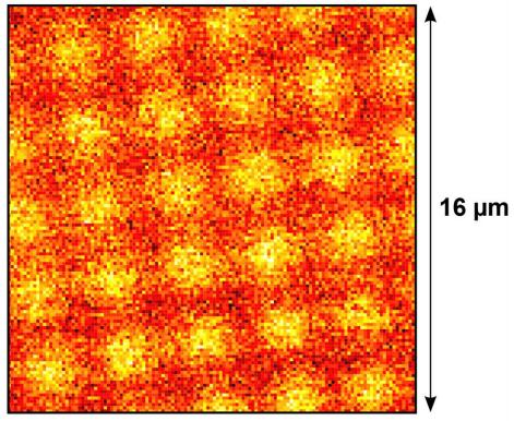
2D images of  $B_{\perp}$  close to the sample surface
