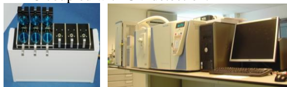
Figure 1: \mu -chamber Figure 2: Thermal Desorption-GC-MS setup
