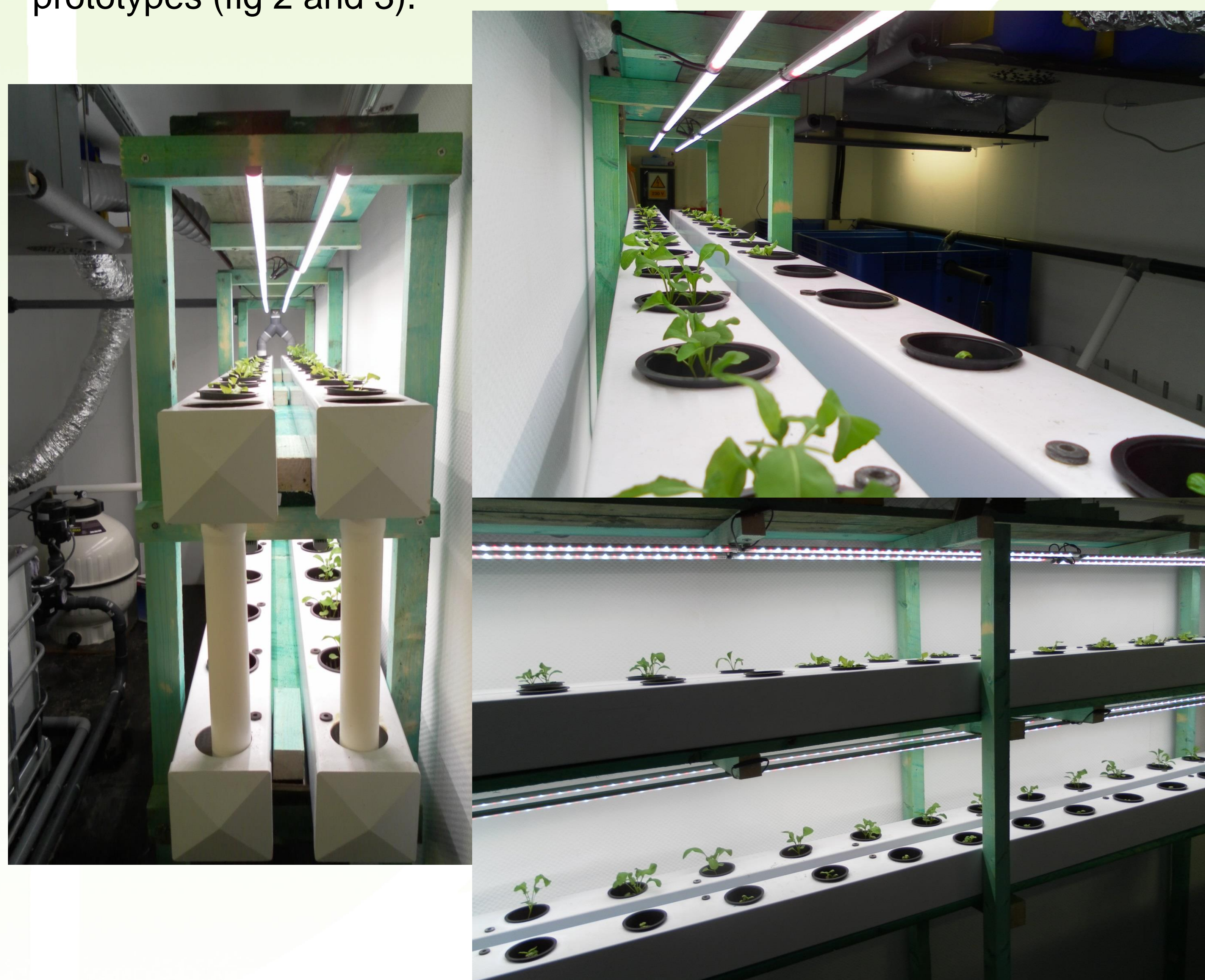
Fig 3. PAFF Box, aquaponic prototype at phytopathology laboratory. NFT lighted by LED technology
