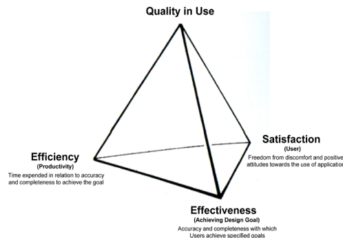
Figure 1 Illustrating the three metrics for measuring the quality of use of CAAD applications. Adapted from (Pak and Verbeke 2011) and (ISO/IEC 25062, 2006).
