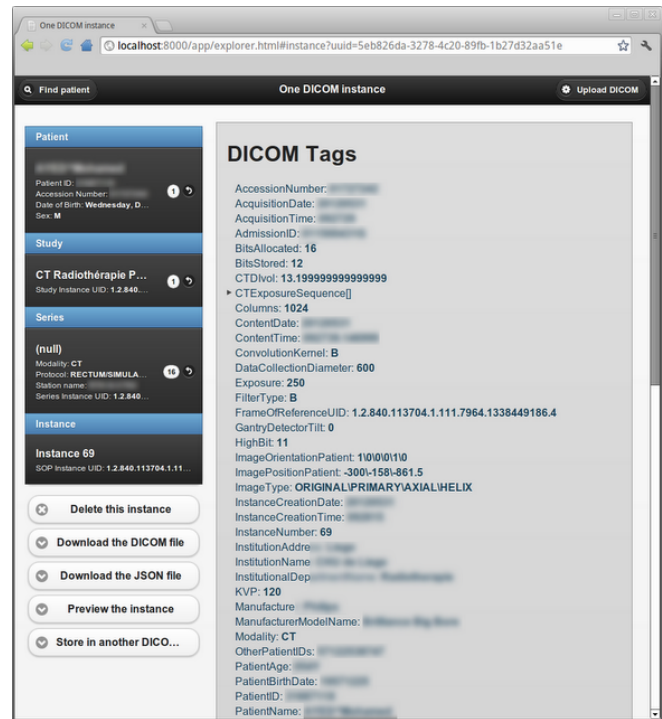
Fig. 3. Displaying some DICOM instance. The right column displays the hierarchy of the DICOM tags. The left column displays the Patient/Study/Series/Instance organization. It is possible to delete the instance, download the raw DICOM file, download a JSON file containing the DICOM meta-data, preview a PNG image, or send the instance to another modality.
