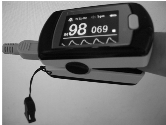
Figure 7.4: The CMS50E finger mounted pulse oxymeter.
